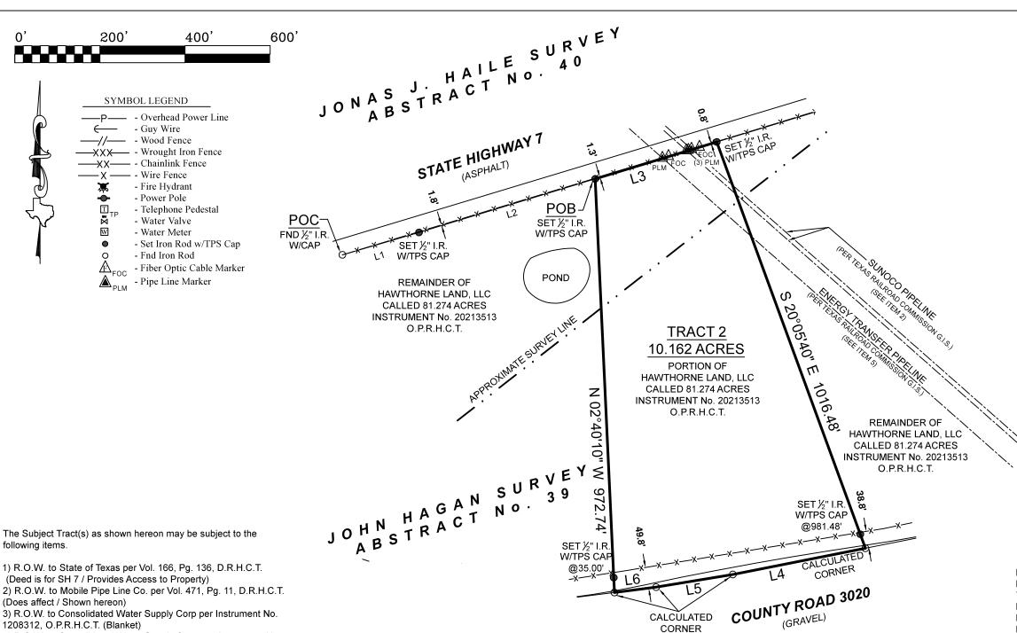
**BEARING** N 73°42'02" E 187.48' 432.44' N 73°05'28" E N 73°05'28" E 298.61' S 78°49'04" W S 80°35'24" W 317 46' 182.57' S 82°43'29" W 98.88'
