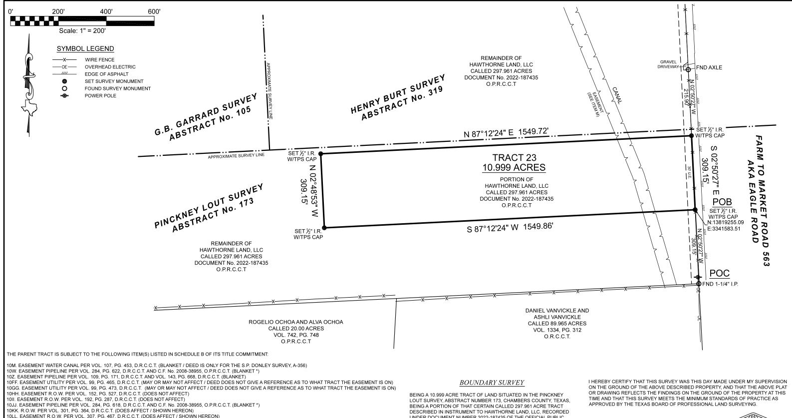
10MM. EASEMENT R.O.W. PER VOL. 320, PG. 418, D.R.C.C.T. (DOES NOT AFFECT) 10RR. EASEMENT PIPELINE PER VOL. 188, PG. 849, O.P.R.C.C.T. (BLANKET \*) \* NO EVIDENCE OF PIPELINES ON THE GROUND AND THE TEXAS RAILROAD COMMISSION GIS DOES NOT SHOW ANY PIPELINES ON THIS PROPERTY) 27332\_TR23 PROJECT NUMBER DATE
